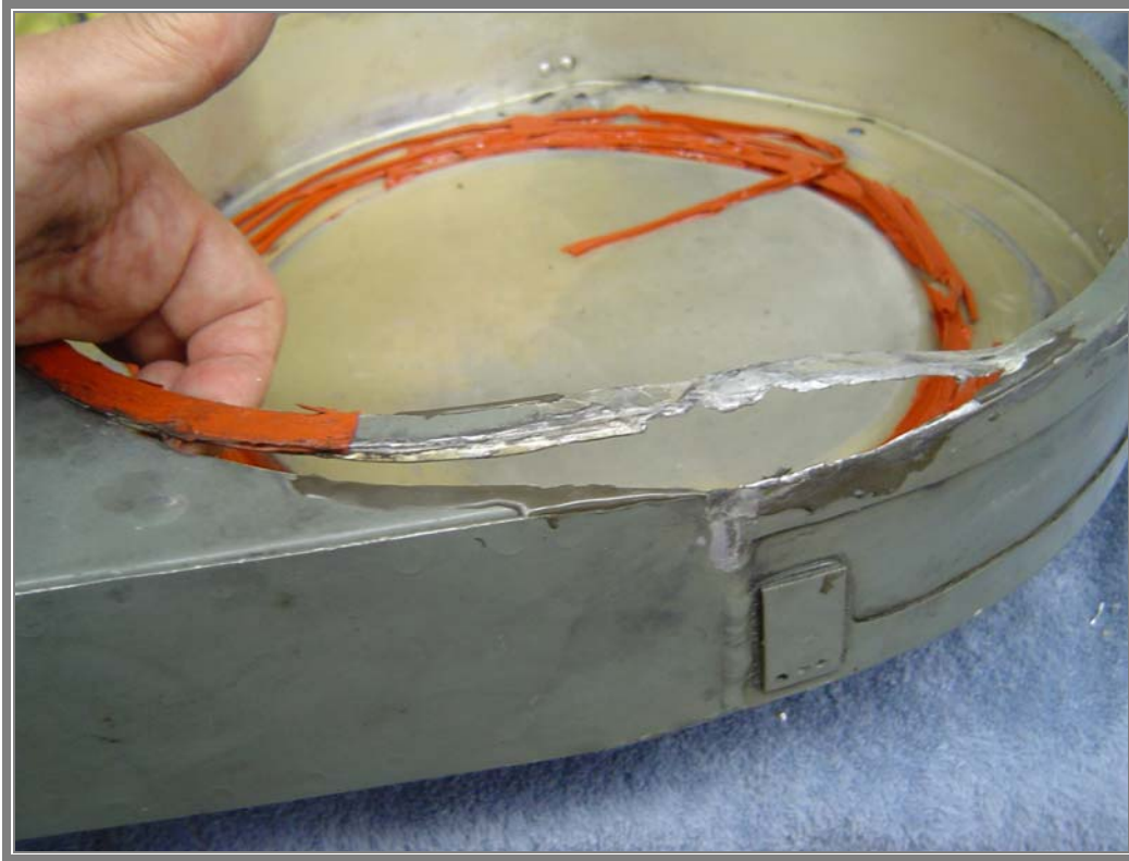
24568-000 BOX ASM, AS RECEIVED. NOTICE THE PRIOR "REPAIRS" USING EPOXY AND SILICONE
