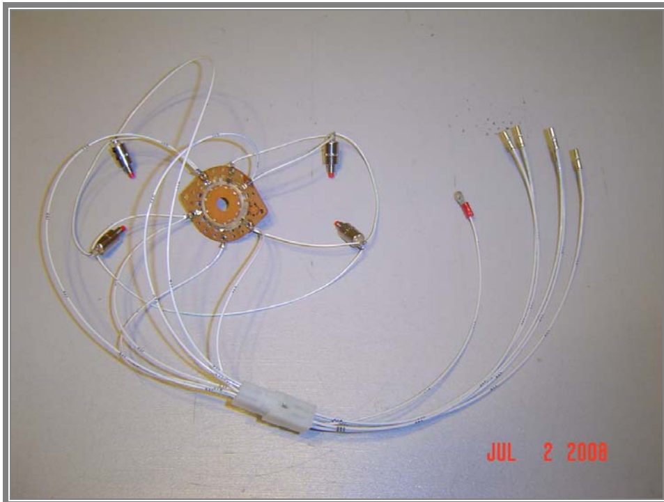
NEW FUEL SELECTOR SWITCHES ASSEMBLY
