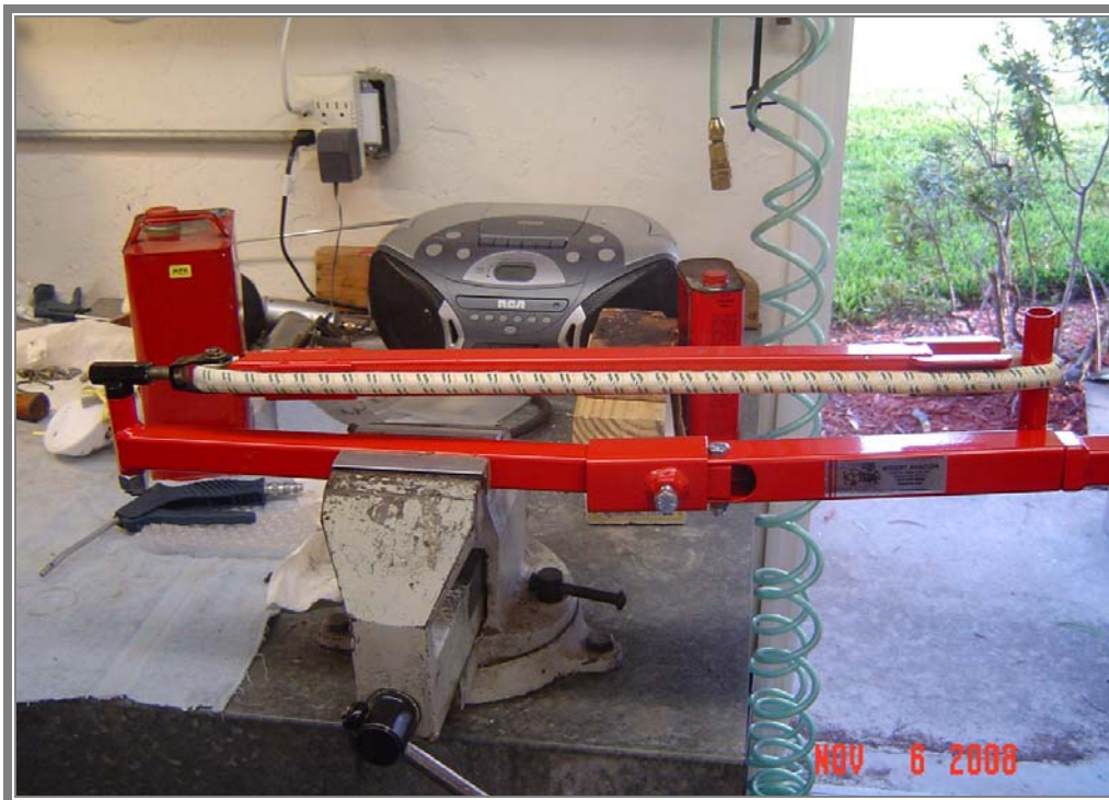
ANOTHER BUNGEE TOOL VERSION FROM BOGERT AVIATION. YOU'LL NEED A ROCK-STEADY VISE ATTACHED TO A HEAVY BENCH TO USE THIS.
