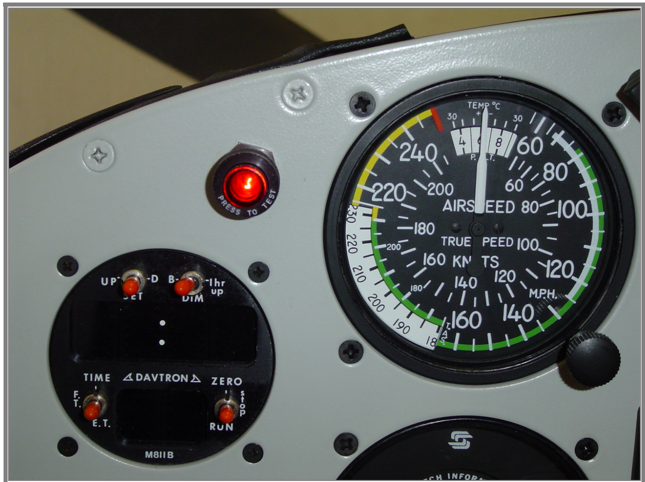
INDICATOR LIGHT INSTALLED IN RON AND JOHN'S STC'D Comanche PANEL
