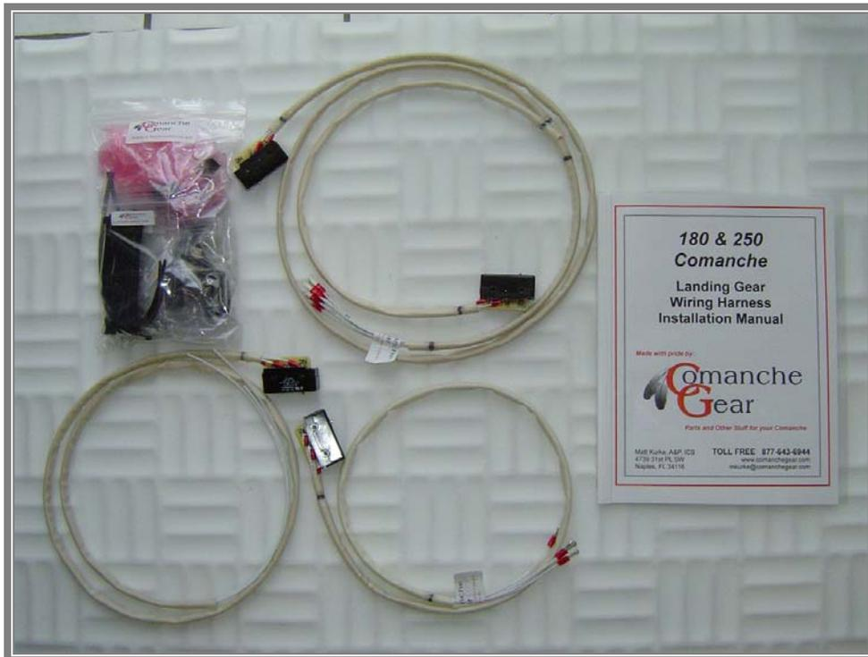
**LANDING GEAR WIRING HARNESS KIT.**
