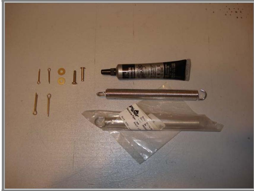
**\$45.00 BASIC KIT CONTENTS FOR REPLACING THE MLG ASSIST SPRINGS.**
