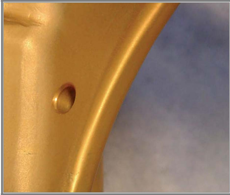
**RADIUS AND POLISH THE EDGE OF THE WEB, AND CHAMFER AND POLISH THE HOLE EDGES AS SUGGESTED IN THE “COMANCHE TIPS”; REFER TO THE PREVIOUS PAGES.**
