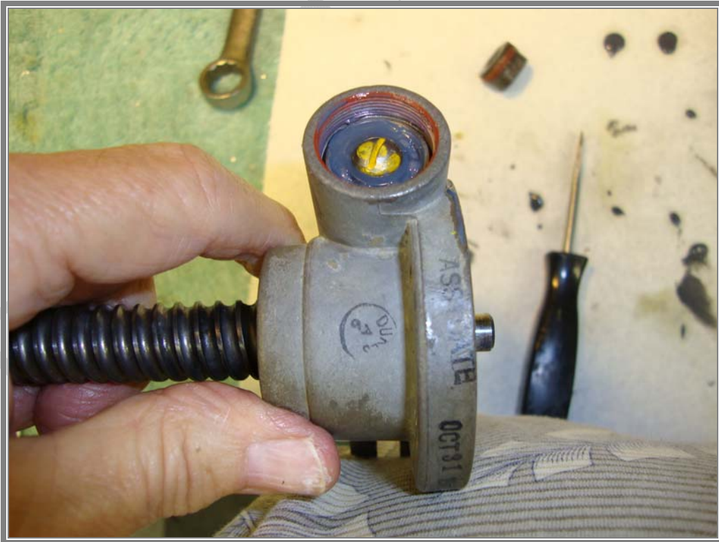
NEW BEARING AT DRIVE SHAFT.
