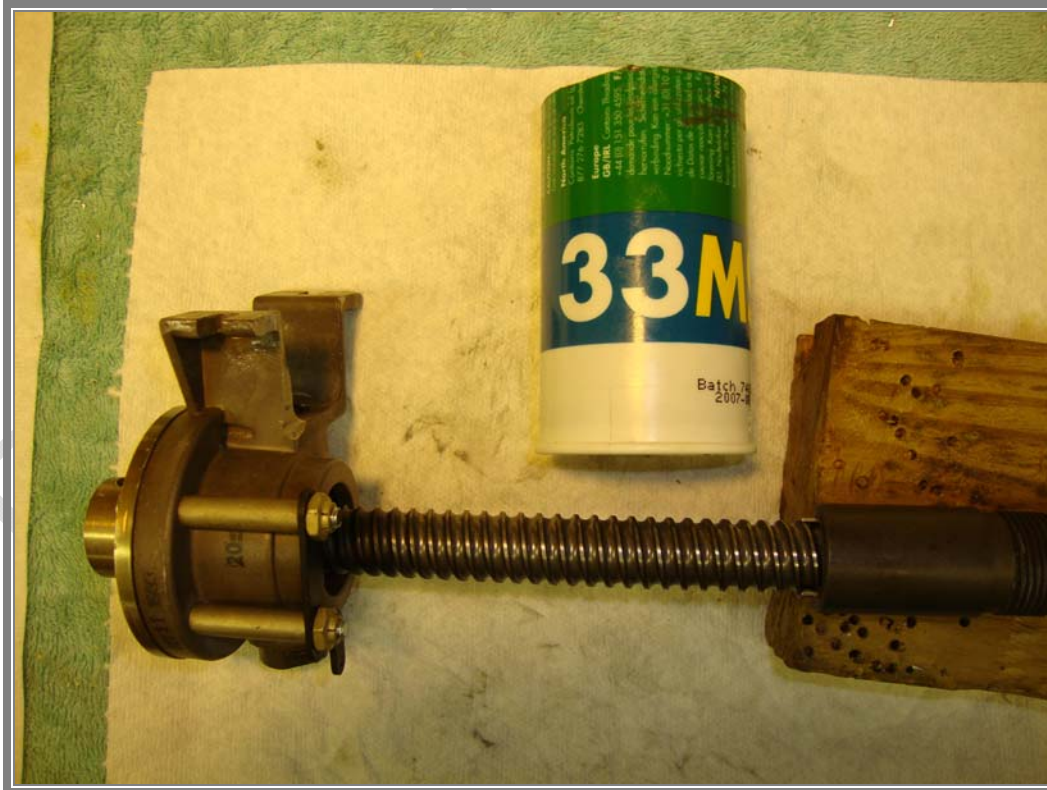
TRAVERSING NUT INSTALLED ONTO JACK SCREW.
