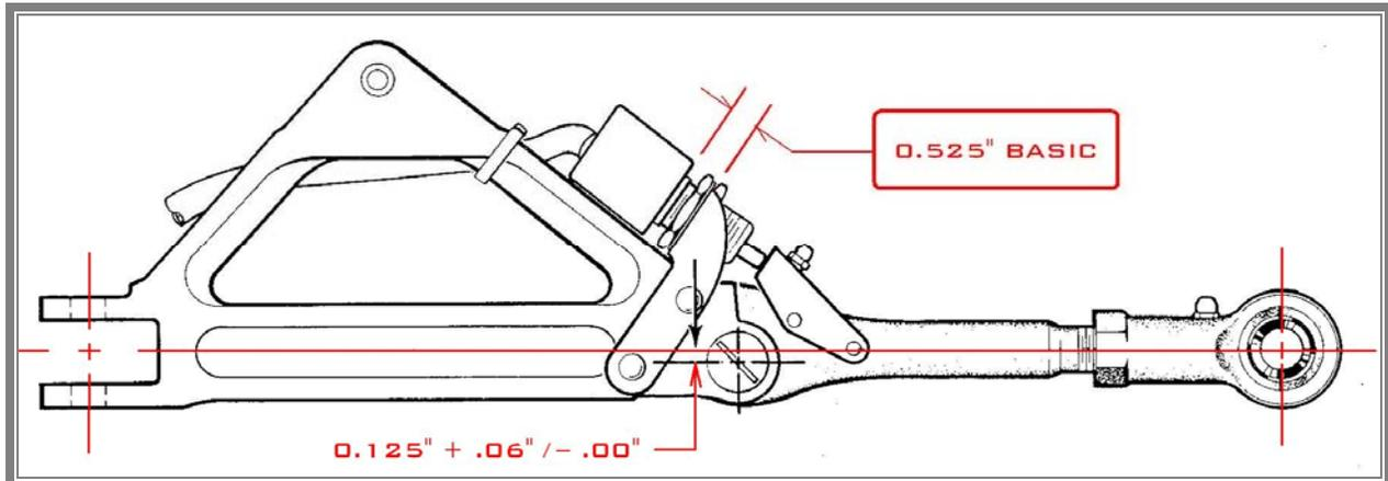
THE DIMENSIONAL METHOD OFFERED HERE CONCERNS THE ROUND VERSION MICRO SWITCHES ONLY – THE RECTANGULAR VERSION DESIGN DOES NOT LEND ITSELF TO SUCH A DISCRETE METHOD BECAUSE THE MOUNTING BRACKET AND STRIKER PLATE CAN BE BENT; HOWEVER THE THEORY IS THE SAME. KEEP IN MIND MANUFACTURING TOLERANCES WHEN CONSIDERING MY DIMENSIONS AND MEASUREMENTS; THERE COULD BE VARIATIONS BUT THEY WOULD BE ONLY SLIGHT. USE THESE SUGGESTIONS WITH THAT IN MIND.
