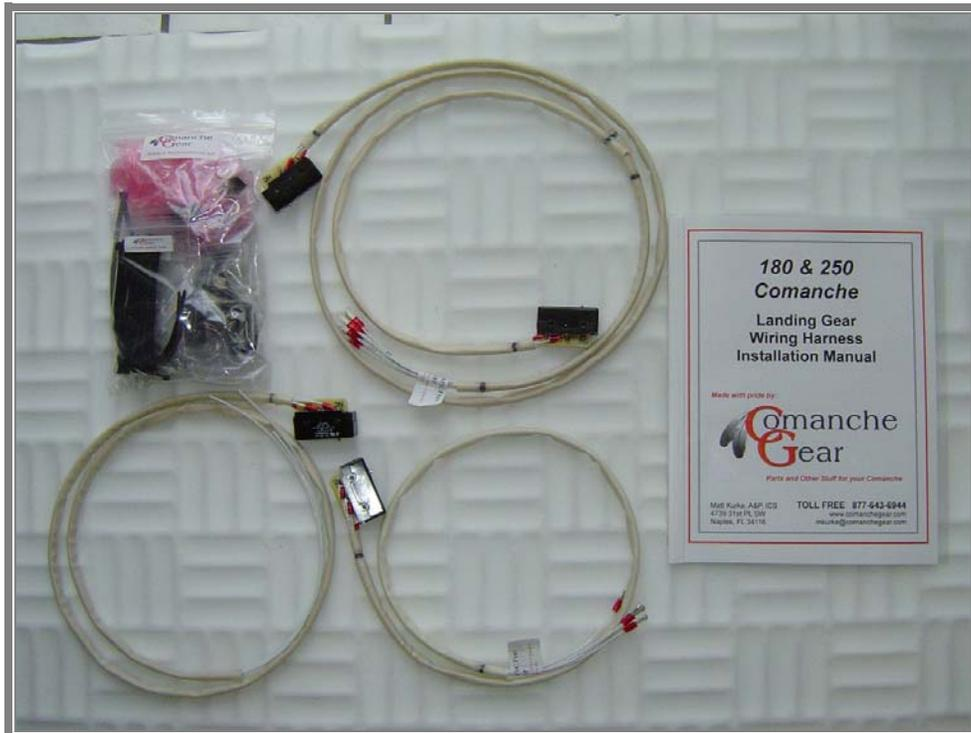
LANDING GEAR WIRING HARNESS KIT.
