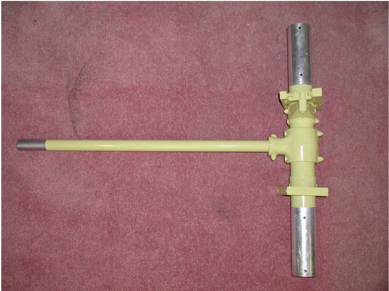
Stabilator Torque Tube Assembly after overhaul and paint
