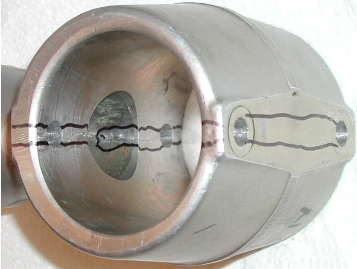
View #2 1958 Comanche 250 3540 hours. Crack visible from outside
