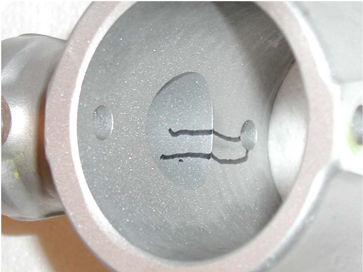
1962 Comanche 250, 3800 hours. Crack not visible from outside.
