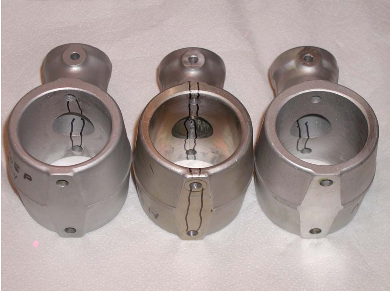
Three cracked horns out of six checked in 2006 Only one crack visible from outside
