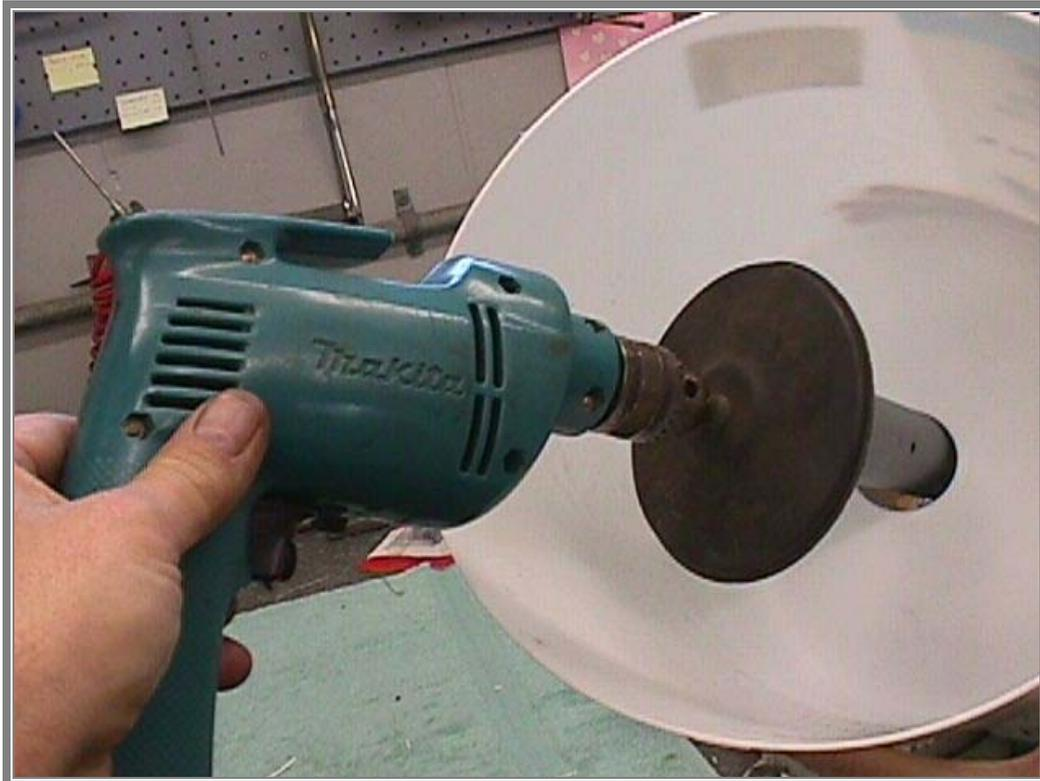
**SETUP FOR SHORTENING THE COLUMN TUBE IF NECESSARY**
