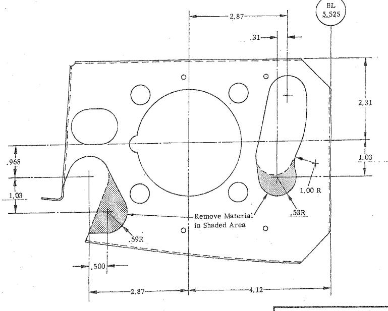
NOTE: Rework existing fuel pump support bracket by enlarging the two cutouts as shown.
